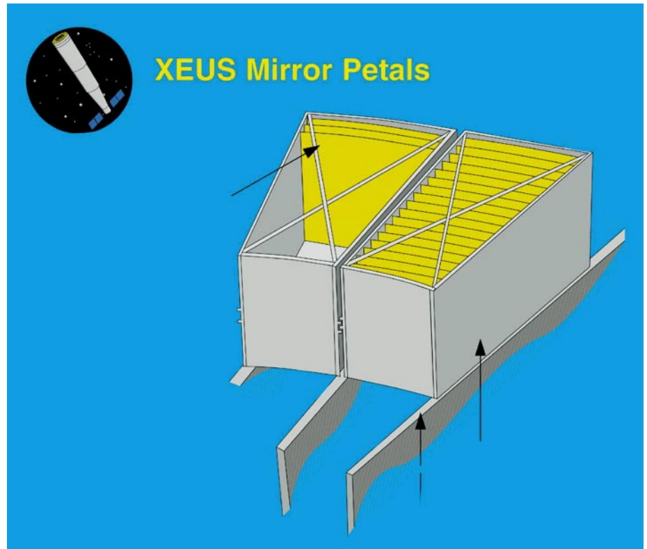
Figure 4.5.1.1. A schematic diagram of a pair of XEUS mirror petals before integration into the mirror assembly structure.
